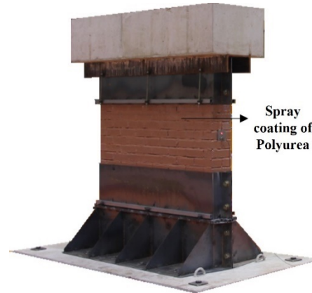
STPU 2mm strengthening MWP2 type- 2 specimen
