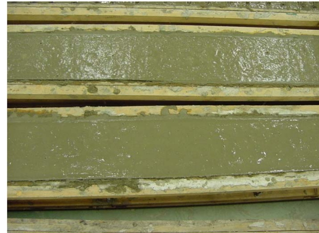
DFRCC Repaired Specimens
