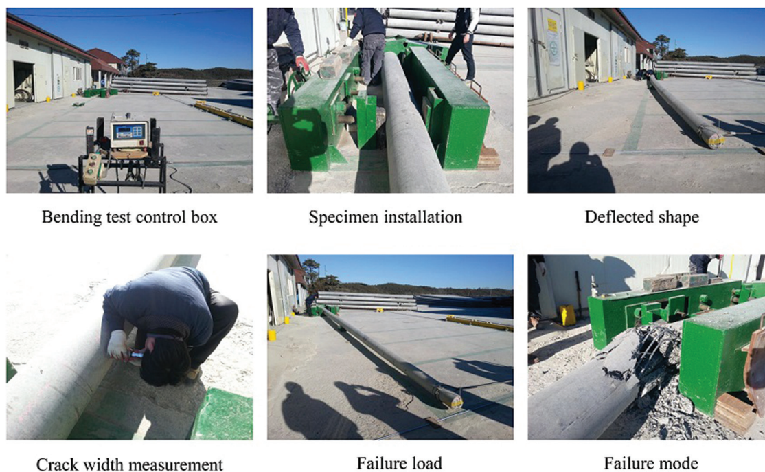
Fig. 4. Photos from bending pull test. [Colour online.]
