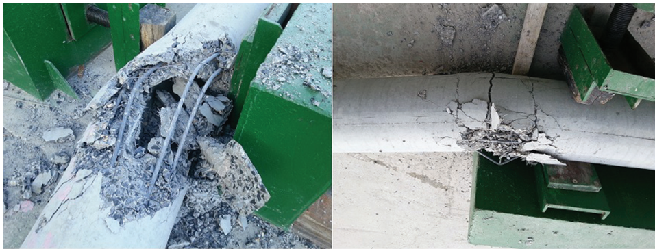
Fig. 9. Comparison of brittle and ductile failure behavior: (a) current EPS and (b) new EPS. [Colour online.]
