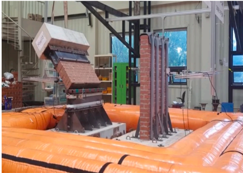
(a) shaking table test photo
